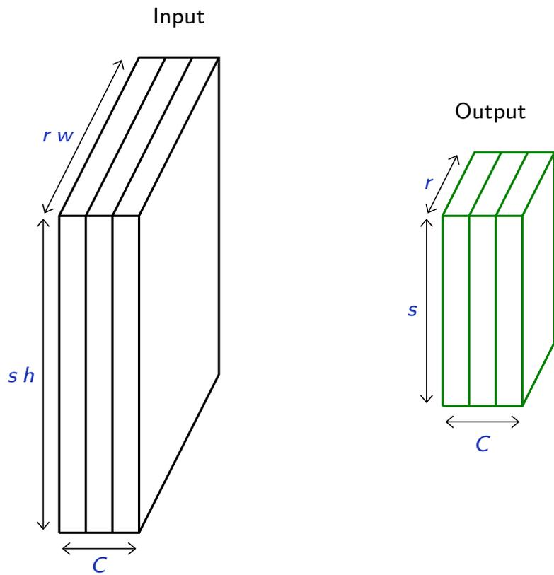
Pooling with a  $w \times h$  kernel. Contrary to convolution, pooling is applied independently on each channel. There are as many channels as output.
